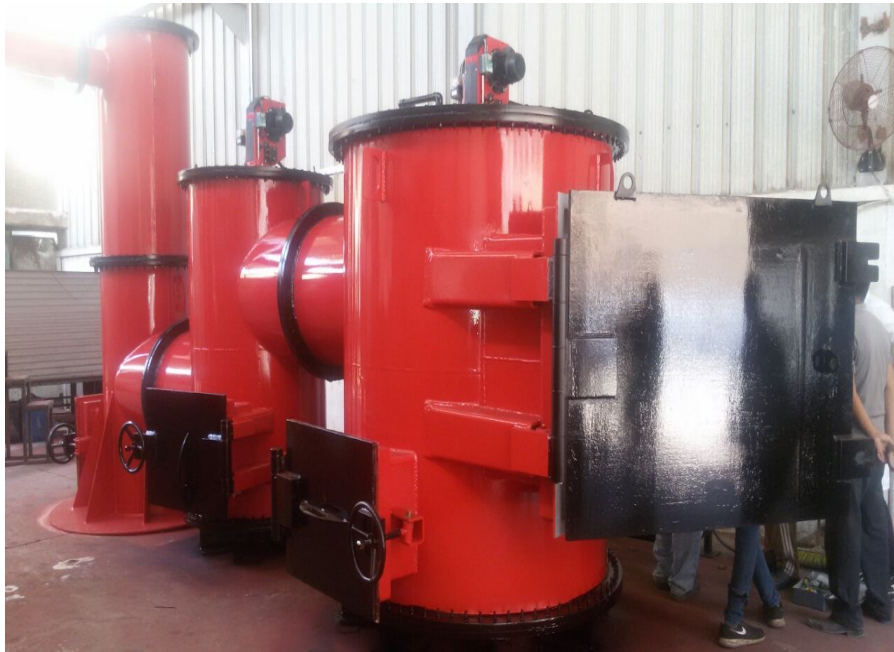
Secondary Combustor/ After Burner
